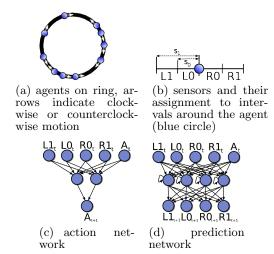
Figure 1: Setup of the collective system, sensor setup, action network, and prediction network [7].
