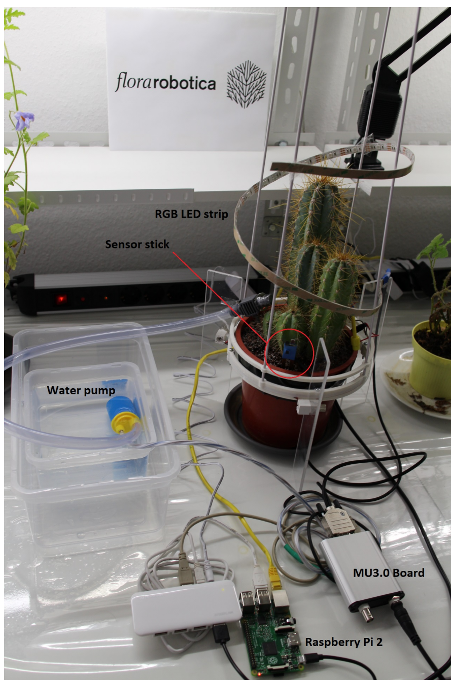
Figure 9: Example system with the main board Raspberry Pi2, the sensor/actuator node (large “electronic fruit”) with MU3.0 and several environmental sensors/actuators.
