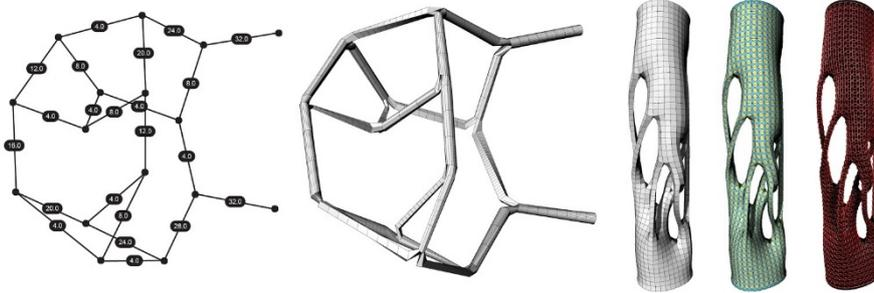
**Fig. 10.** Example mesh solution (center) from a weighted macro scale directed graph topology (left) and the eventual result from the braid solver (right).
