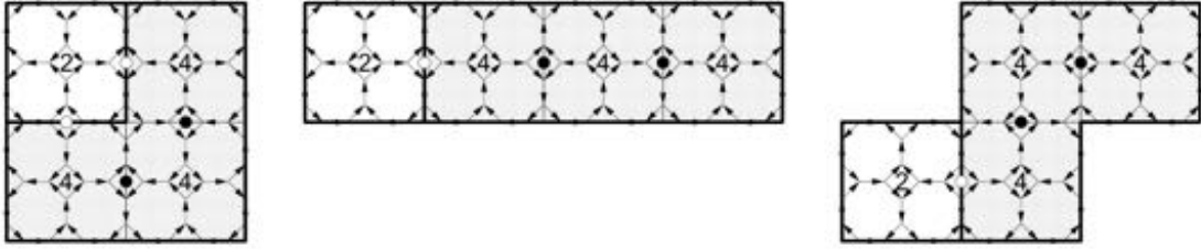
Figure 18: Same horn gear neighborhood connectivity for three geometric machine variants.
