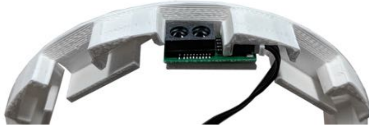
Figure 52: 3D-printed case cross-section showing the mechanical anchoring of an IR-proximity sensor around the circumference of the robot node. The ten IR sensors are the primary components requiring mechanical anchoring in the case, as other components are mechanically affixed to the PCB and heatsink.
