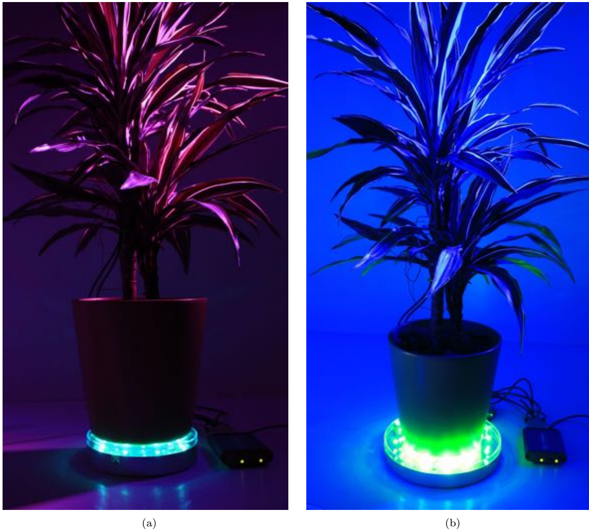
Figure 46: Interactions with users via color indication: (a) low-intensity RGB light base 6 inch; (b) middle-intensity RGB base 8 inch.
