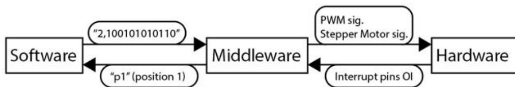
Figure 2: Direction of messages passed between software, middleware, and hardware.
