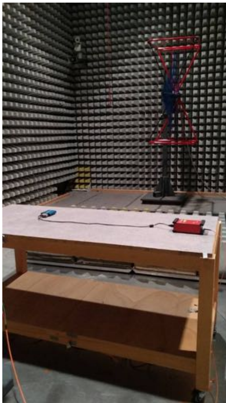
Figure 43: Tests on electromagnetic compatibility of the phytosensor system in the SGS Germany GmbH (Munich) certified laboratory: test on EM immunity.
