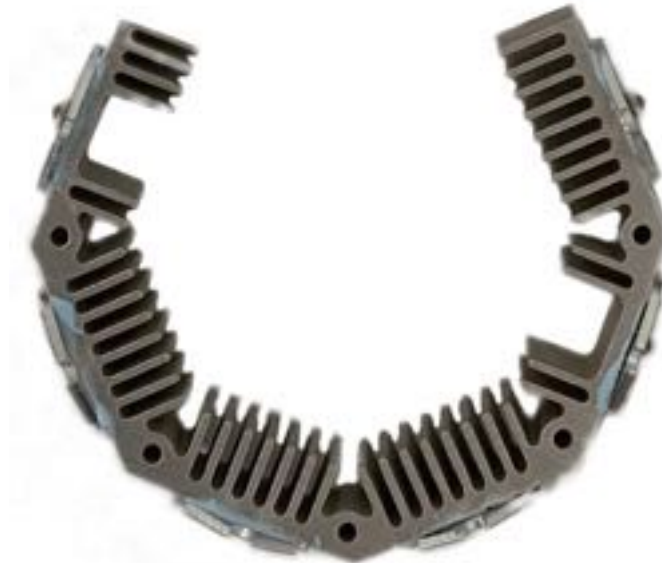
Figure 53: Custom waterjet cut aluminum heatsink. Six LEDs are affixed to the six faces of the heatsink using thermal adhesive.
