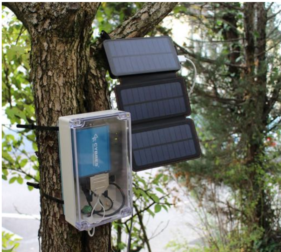
Figure 36: Outdoor setup with solar cells and WiFi data transfer
