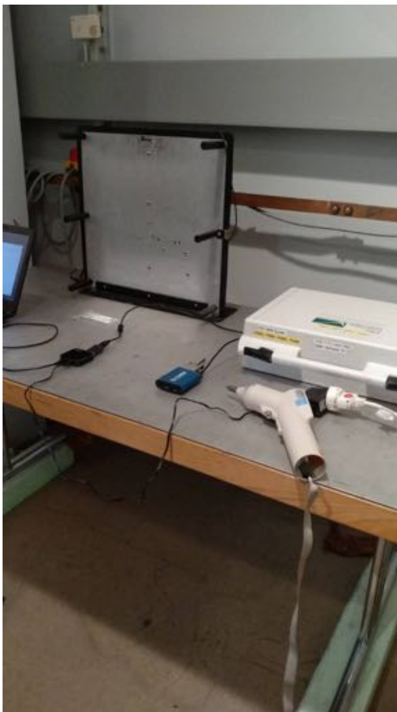
Figure 44: Tests on electromagnetic compatibility of the phytosensor system in the SGS Germany GmbH (Munich) certified laboratory: test on electrostatic discharge immunity.
