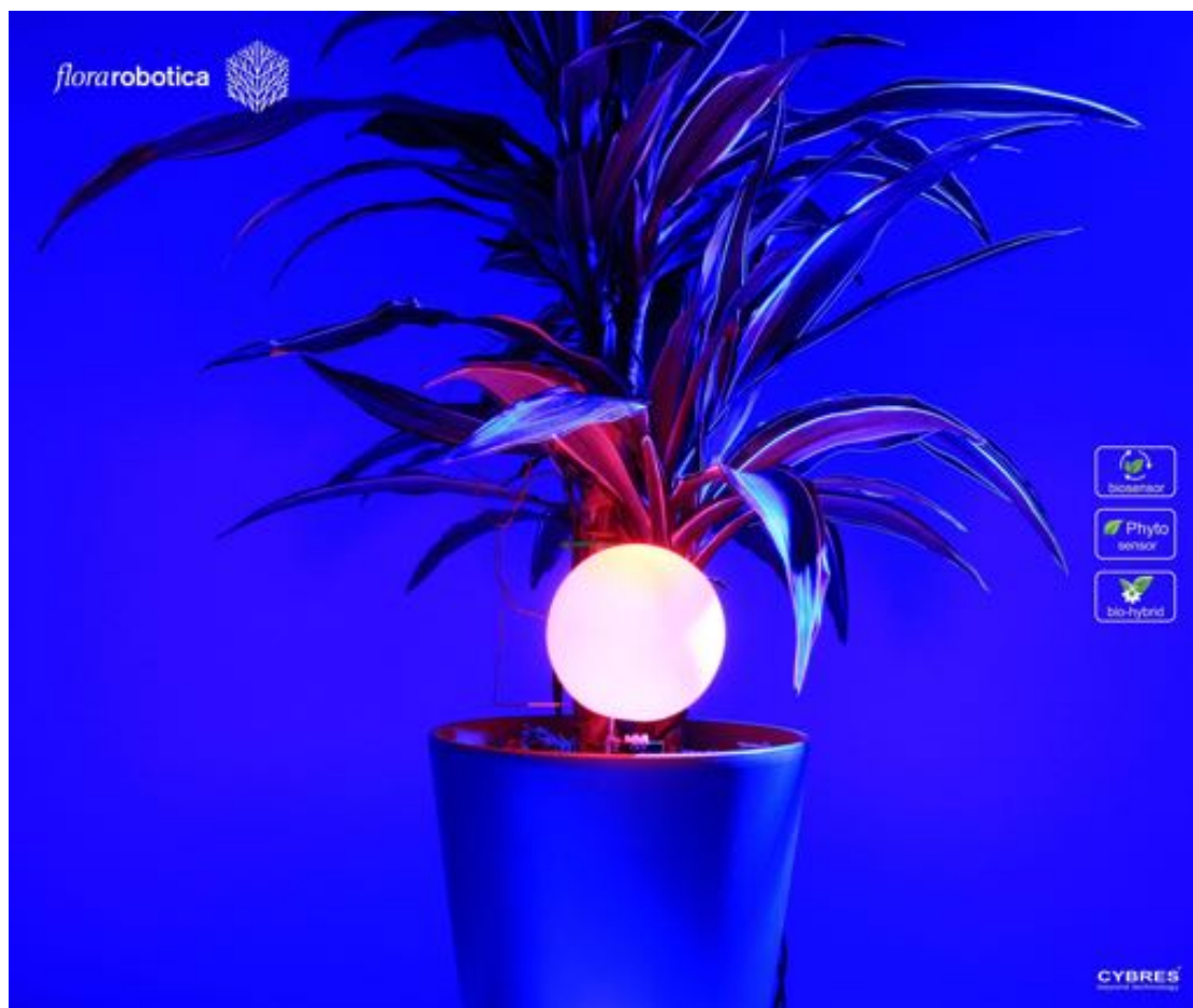
Figure 45: Interactions with users via color indication: low-intensity RGB light ball.
